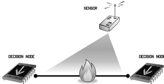
Figure 1. A sensor node (SN) monitors a graph edge for possible hazards. In the IES, decision nodes (DNs) located at graph vertices receive measurements from their adjacent SNs and provide dynamic directions during evacuation.
