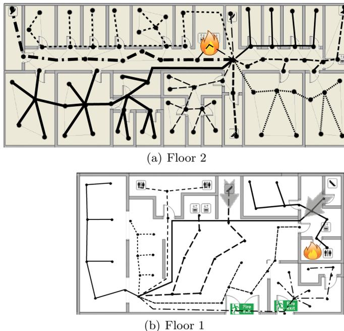
**Fig. 1.** Floor plans of the building simulated, showing the sensor nodes (black dots) and the network layout, and the initial fire locations in different simulations (flames).
