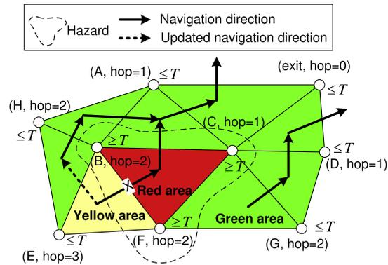
Fig. 3. An example of area-to-area navigation paths. (For interpretation of the references to colour in this figure legend, the reader is referred to the web version of this article.)
