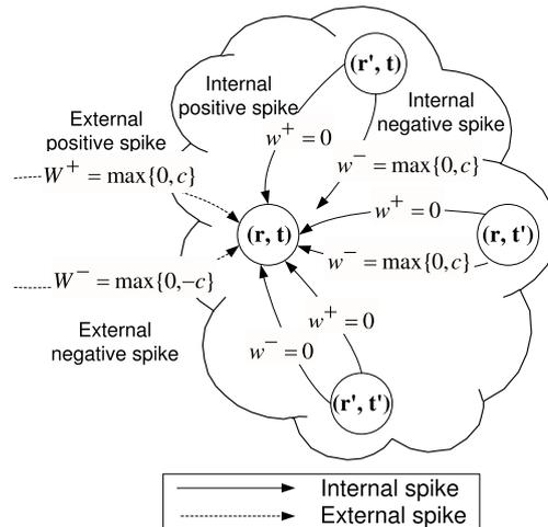
Fig. 6. The model of RNN for the resource allocation problem.
